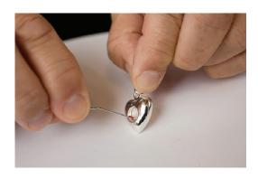
5. Rub the Loctite® paper clip around the threads.
